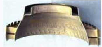
Low distortion of LENS process allowed this part to be salvaged
